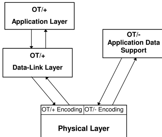
The **Application Layer** is responsible for transfer of application data between the application software in the boiler and room controllers. It defines data-classes, data-id numbers and format of data-values for transmission. It also specifies the minimum AL support for all OpenTherm-compatible devices.
