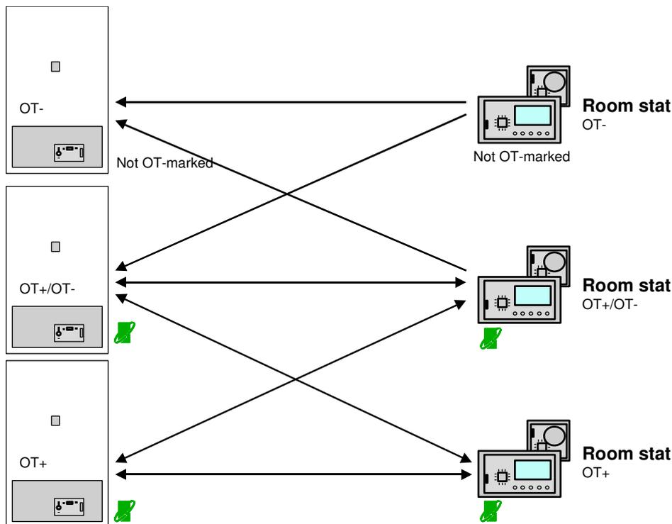
When a room unit which can operate both in OT/+ and OT/- modes is connected to a boiler controller, some configuration needs to take place to determine which protocol to use. This configuration should be achieved automatically as follows :
