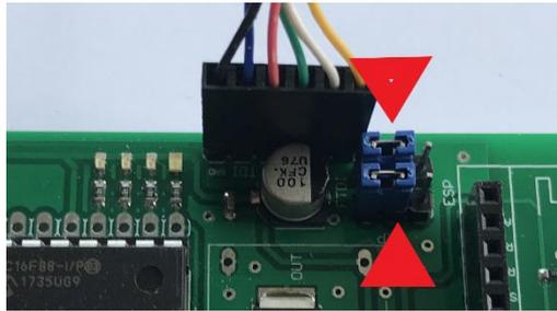
With a cable with 4 separate connectors, only the black, green and white wires must be connected. The connector with the red wire is not necessary.
