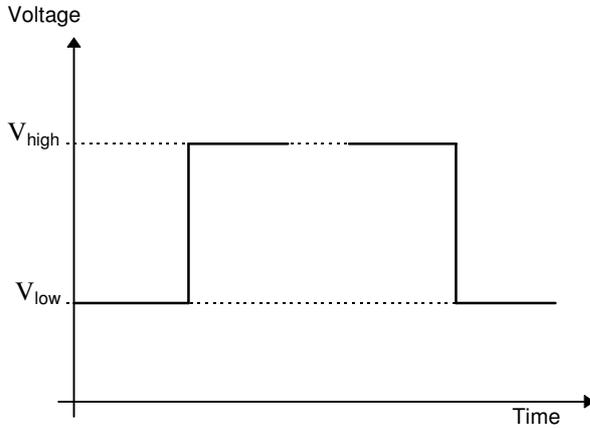
Voltage signal High level       $V_{high}$       :      15 .. 18 V.
