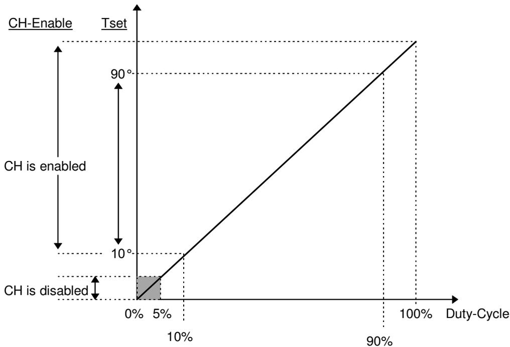
The tolerance of both generation and measurement of the Duty-Cycle signal should be less than  $\pm 2\%$ .
