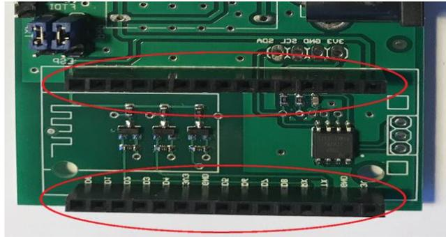
**For USR-TCP232-T2:** Cut down the 2x15 female header strips and solder to the positions shown.
