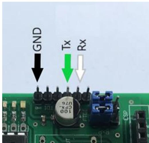
With an FTDI board, GND on the board connects to GND on the gateway.
