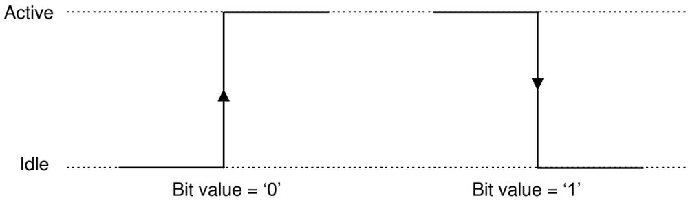
Manchester encoding is a self-clocking code giving the advantage of bit-synchronisation since there is always at least one transition in the middle of the bit-interval. It also has a fixed average d.c. component over the frame of half the idle and active levels which allows greater predictability of power supply requirements, and additionally the absence of an expected transition can be used to detect errors.
