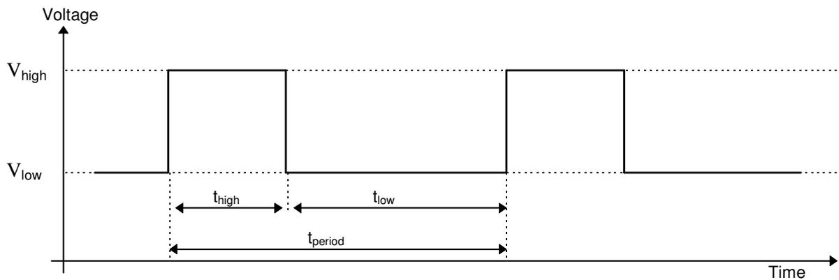
Duty Cycle (%) =  $t_{low} / t_{period}$  ie. the % time over the period that the line is **low**.
