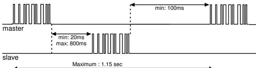
A conversation is limited to a single exchange of frames. Three types of conversation are possible, listed in the next section.
